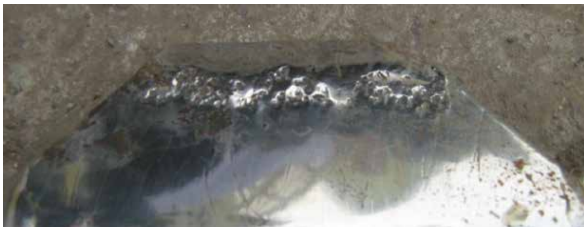
Fig. 14. Typical view of the friction surface of the working body hardened by EDM
