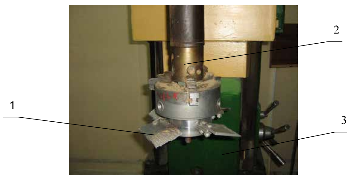
Fig. 6. Shaft holder with prototypes: 1 – prototype; 2 – shaft holder; 3 – 2E78P machine
